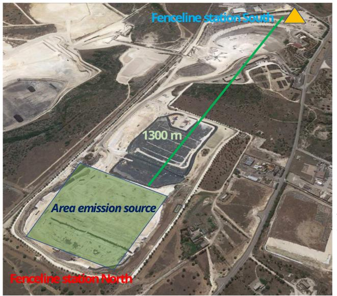
Non hazardous waste landfill; mostly sewage sludge and wastes deriving from mechanical-biological treatment of
